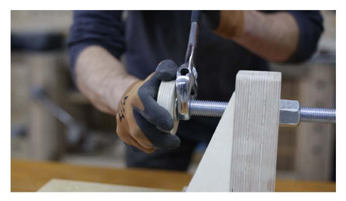
Now I make a hole in the third piece using a bit with the same diameter as the threaded rod. At this point I can glue the three pieces. I machine and screw in these reinforcements. I attach the handle which I've drilled with a bit with 1mm less diameter than the threaded rod.
