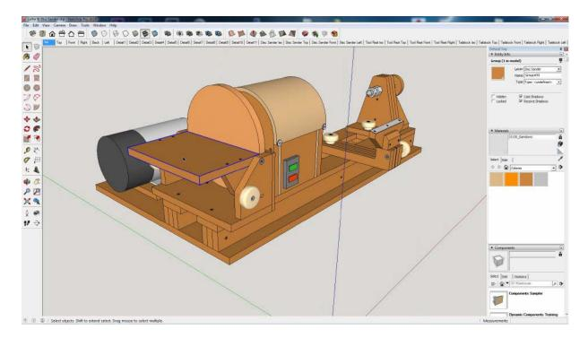
As you can see, I've also attached a **Disc Sander** on the left side to take advantage of the motor's rotation. This is the disc sander's stand, which can be tilted up to 45°, which will definitely come in handy sometimes!
