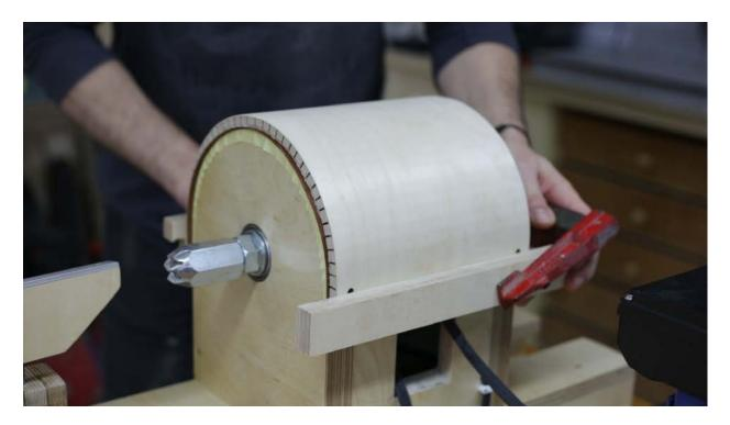
I fill all the holes with glue. I use glue on a 0.4mm thick veneer of any kind of wood, and put it in place with the help of these plywood pieces and clamps. Ideally, for this kind of operation we would have a mould and countermould, but with this method we can also achieve decent results.
