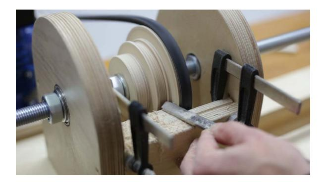
Now I'll machine the lathe's pulleys attaching them to the motor, and I'll take the chance to see if everything is working correctly. These pulleys must be of the same diameter as their motor counterparts so that we can change between them without having to move the motor.
