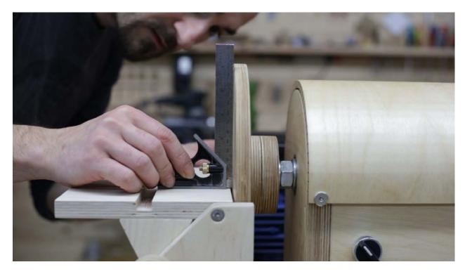
I mark the holes for the screws that will serve as rotation axis. In this case I will use a drill bit 0.5mm less wide than the screw. I make a groove to insert a U-shaped aluminium profile to slide the Miter Gauge on top of. I've machined both pieces that will allow me to lock the table at an angle and screw them in like this.
