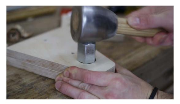
I'll mark the centre to drill a hole with the threaded rod itself. It seems to match the template quite well! I drill a hole in it and press fit this **coupling nut**.
