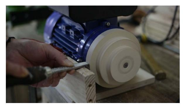
Now it's time to lathe the pulleys. I will start with the widest one.
