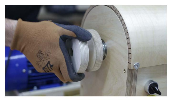
Now I'll start working on the disc sander. I mark its circumference on the board and cut it. I use a bit 1mm less wide than the threaded rod when drilling. By rotating the wooden disc when inserting it, I'll create a thread on the plywood itself allowing me to remove the disc when necessary.
