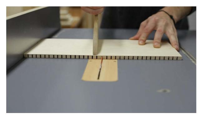
I'll begin by cutting and machining the lathe's cover. In order to fold it, I'll make some cuts on the underside, leaving only 1.5 milimetres uncut. It's important that the grain on the final layer of plywood be perpendicular to the cuts, so that it won't break when folding.
