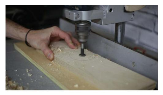
These are the motor pulleys. I've drilled holes in them with the exact diameter of the motor shaft.
