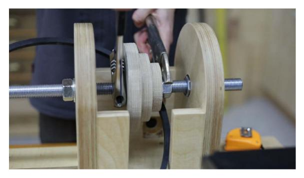
Before we move on, I insert the belt. I place all the nuts and washers, check the measurements, and now I can fasten and screw everything in place.
