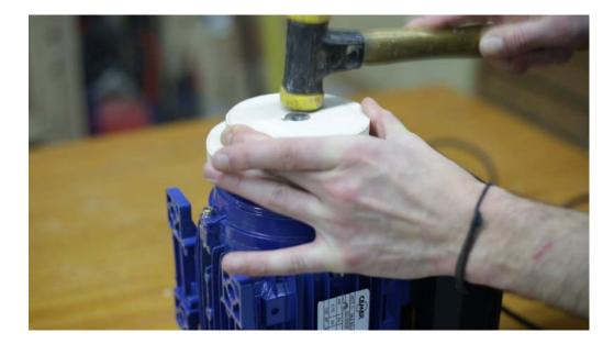
After machining the pulleys, we insert them in the shaft being careful not to hit them too hard to avoid damaging the motor. Then, I place a screw in front of axis to hold them.
