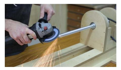
Using an angle grinder I sharpen the threaded rod.
