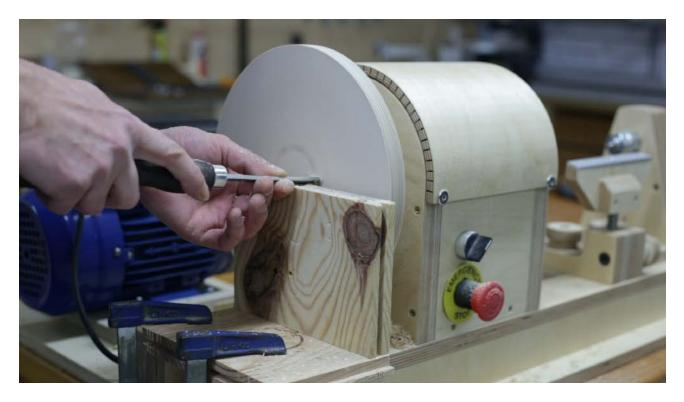
I will lathe all the pieces to reduce any potential vibrations. Also on the front of the disc, to avoid oscillations and make it run smoothly and then I'll sand the edges of the disc for safety reasons.
