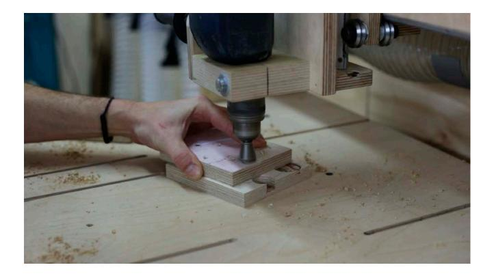
I'll start machining all the pieces of its tilting table. The disc must be removable for when we lathe at high RPMs. If we don't remove it, the vibrations could be excessive for lathing due to the diameter of the disc itself. Therefore, I'll use the same fastening system I used for the tailstock and tool rest allowing me to easily remove the tilting table and disc.
