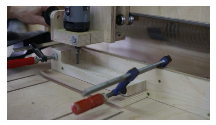
Now I machine the pieces for the toolrest and glue them together like before. With the **3D Router**, I machine this fitting groove. I make a hole here to insert a piece of threaded rod that will allow me to adjust the height of the toolrest.
