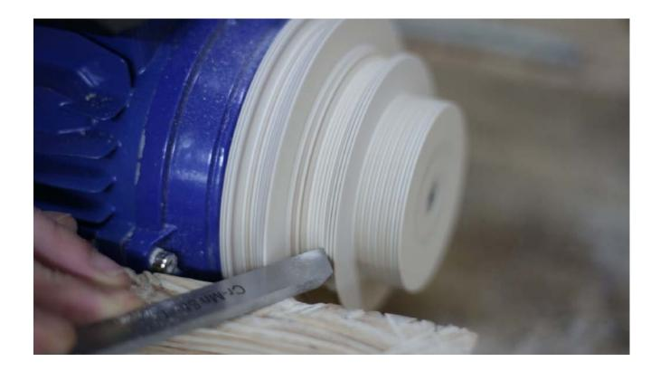
I'll lathe the groove for the **V-belt**, I'll try it little by little to adjust it correctly.
