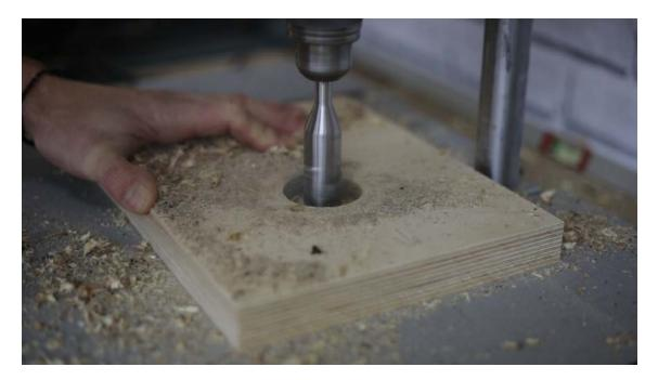
Once dry, we create a place for the bearings with an **adjustable drill bit**. I will drill the hole at low RPMs, advancing slowly to avoid burning the wood and the bit.
