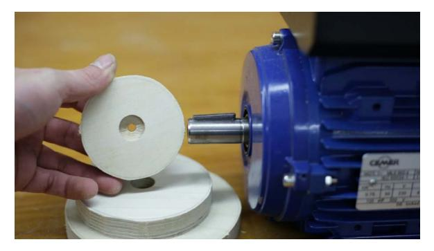
As you can see, the shaft has a slanted part that sticks out that will prevent the pulleys from moving backwards, and at the same time will provide traction.
