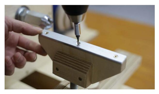
I drill and countersink this piece of aluminium to protect the toolrest. And finally, I'll do a little test with a piece of ash wood. After marking the centres, I put it in place, tighten all the knobs and adjust the toolrest's height. Since it's not a wide piece, I'll select the pulley combination with the most RPMs. Seems everything's working as it should! It runs smoothly, without vibrations, and the drive centre isn't slipping off.
