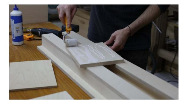
Now I'll attach these two pieces with glue to achieve greater thickness. This is the part where I'll insert the **bearings** that will serve as rotation axis.
