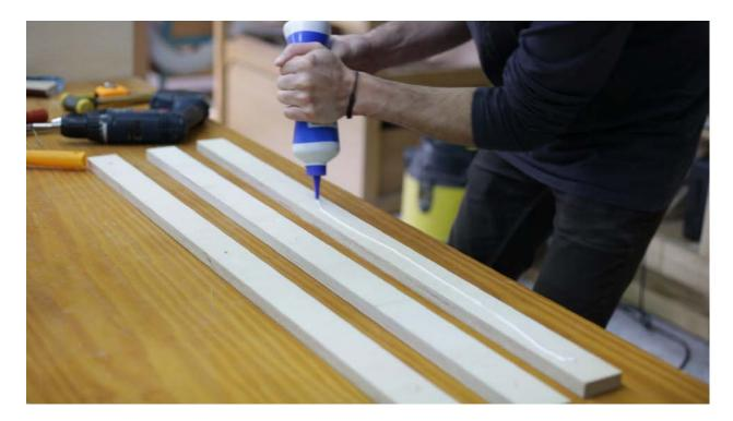
We apply glue on these three pieces that will function as base for the lathe. First I place a couple of screws so that the pieces won't move when fastening them due to the viscosity of the glue.
