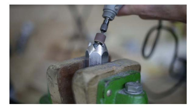
Now I put the motor in place. I'll use two flat hinges to make it turn. I'll use another coupling nut to make the drive centre. Then I mark it like this and cut it with a hacksaw. Now I'll make a bevel with the angle grinder to sharpen the tips. I finish the job with a file and a dremel.
