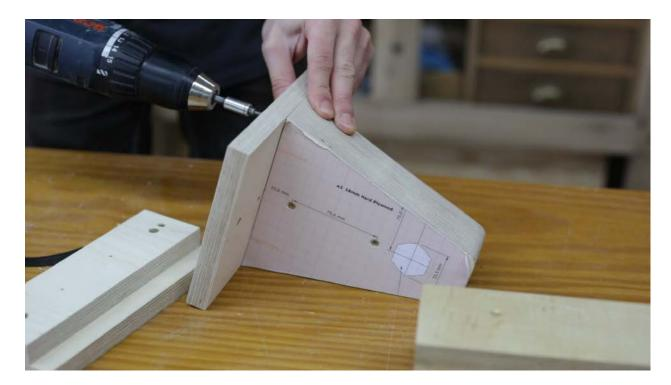
I machine the base and screw it to the three pieces.
