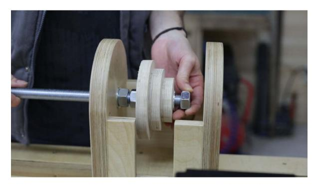
We put the bearings in place and attach the threaded rod. I place the lathe's pulleys and glue them together.
