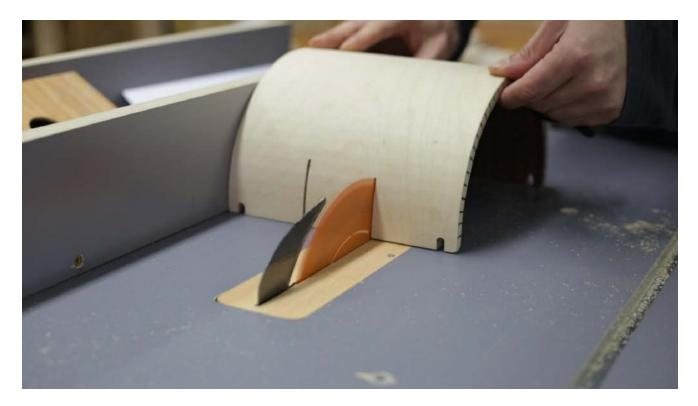
I cut this hole for the belt with the **table saw**. Then I mark the positions of the screws and drill them, I'll use a drill bit 0.5mm smaller than the screws.
