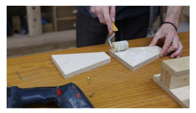
First I'll cut and glue these two pieces for the tailstock. Just like before, I'll use a pair of screws in addition to glue. Now I sand the edges. The third piece will only be screwed in so that it can be removed later.
