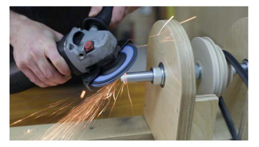
Cut this piece that I will use for the lathe's tailstock, and I do the same sharpen again on this end.
