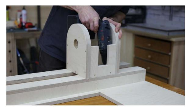
Now I'll screw the set to the base. Having done that, I apply a couple of coats of **spray varnish** now that it's easy, and while it's drying, I'll cut the six pulleys, three for the motor and three for the lathe.
